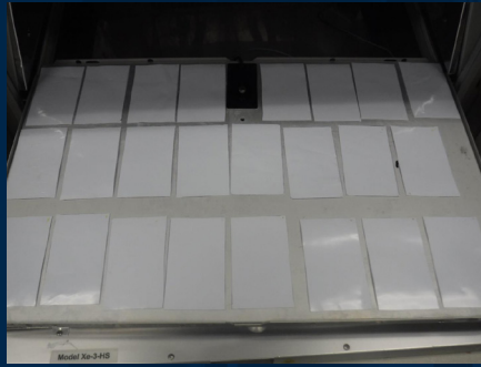
Fabric sample placement for UV Testing
