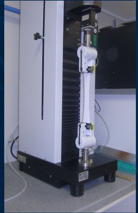
All samples were tested to ASTM D882
