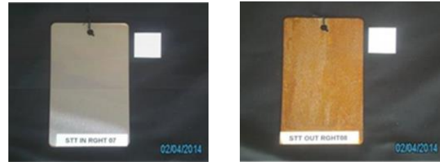
Figure 1. Typical coupon results showing coupons protected by an XT cover and exposed to the environment.
