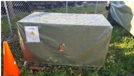
MEP-803A generator protected by an XT cover
