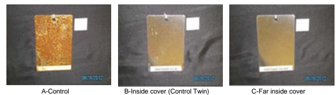
Figure 3. Coupons after six months of natural weathering.
