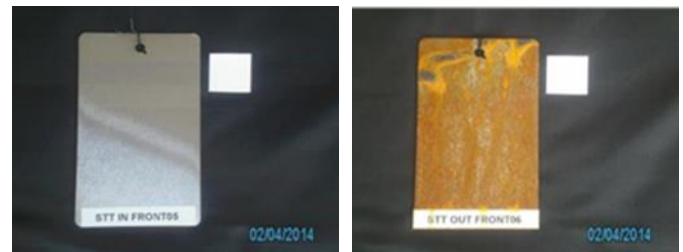
Transshield XT 99.9% Protection Outside Cover 12.3% Protection Figure 2. STT Coupons After Testing
