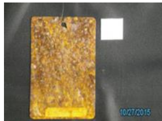
Outside Cover 0.0% Protection MEP-1040 Generator
