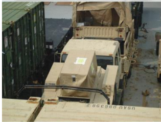
U.S. Army MEP-1040, 10kW 50/60Hz Generator with an ArmorDillo cover
