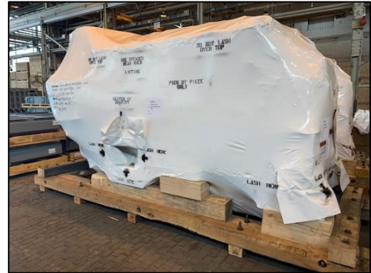
Figure 4 Asset protected by shrink wrap
